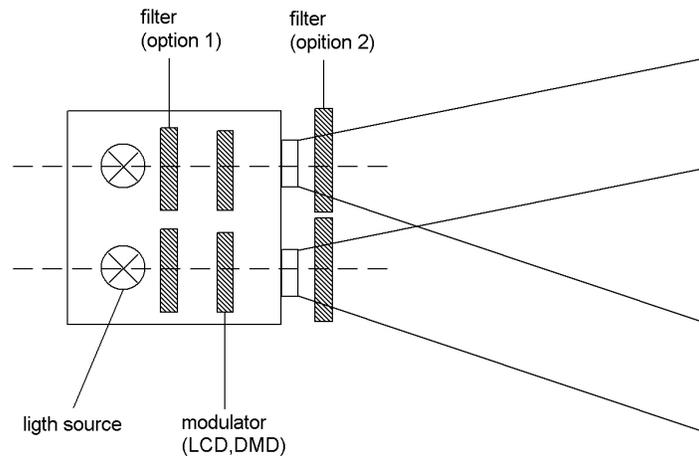
Fig. 4: Schematic set-up of an interference filter technique (Infitec) system for stereo imaging using conventional digital projectors.
