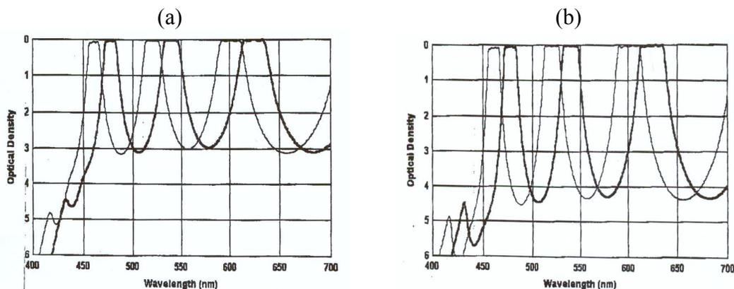
Fig. 5: Triple band characteristics of a three cavity design (a) and of a four cavity design (b).
