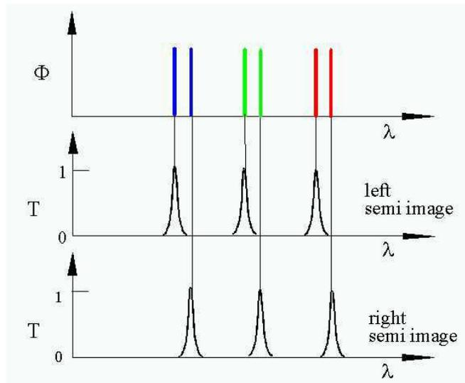
Fig. 3: Stereo imaging using two wavelength triples.
