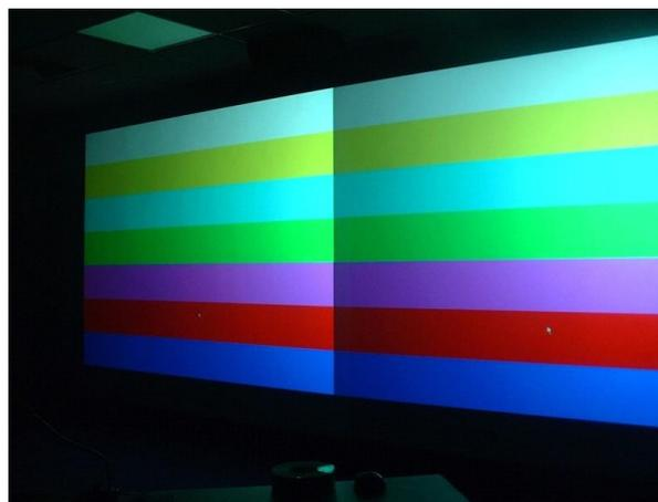
Hard-Edged Image on Non-Depolarizing (Silver) Screen
