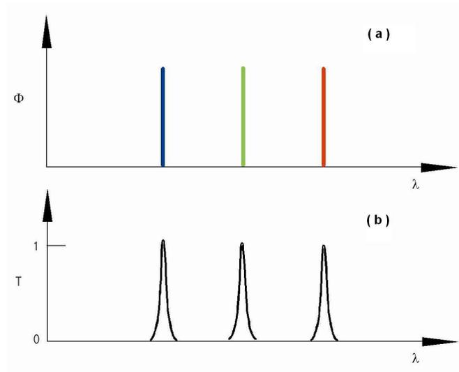
Fig. 2: Spectrum of the image (a) and corresponding filter characteristic on the side of the viewer (b) in narrow band wavelength multiplexing visualisation systems.
